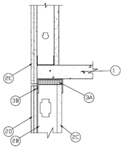
1. **Floor Assembly** — Min 4-1/2 in. (114 mm) thick steel reinforced lightweight or normal weight (100-150 pcf or 1600-2400 kg/m<sup>3</sup>) structural concrete. Floor may also be constructed of any min 6 in. (152 mm) thick UL Classified hollow-core **Precast Concrete Units\*.** See **Precast Concrete Units** (CFTV) category in the Fire Resistance Directory for names manufacturers.
